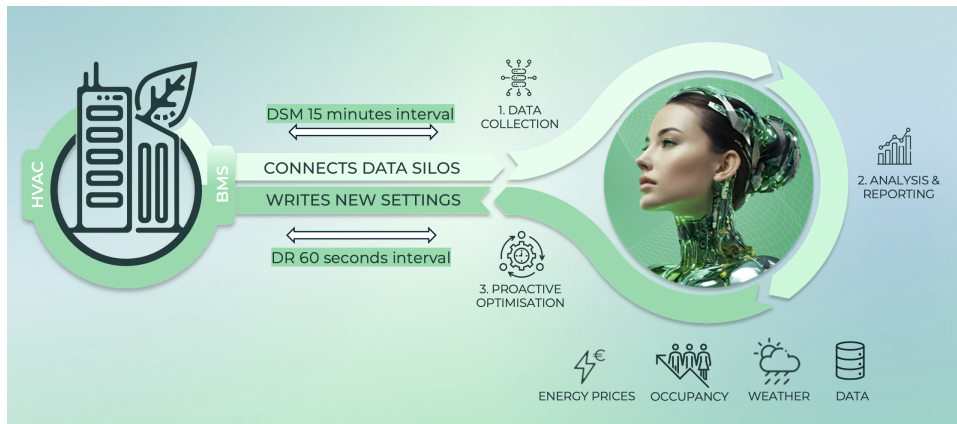
Fig. 1. The general structure of the provided AI-based solution to provide real-time operation of Demand Side Management and Demand Response simultaneously.
